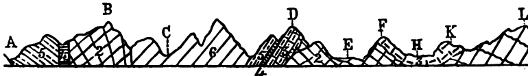
Section (1)—From Hollyford Valley, across Lake Harris Range and Humboldt Mountains, to Richardson Mountains. 1. Crystalline schists. 2. Foliated schists. 3. Lake Harris schists. 4. Cecil and Walter Peak series. 5. Serpentine. 6. Te Anau series. A. Hollyford Valley. B. Lake Harris Range. C. Upper Route Burn. D. Upper Peak. E. Dart River. F. Mount Alfred. H. Rees River. K. Precipice Hill. L. Richardson Mountains.
